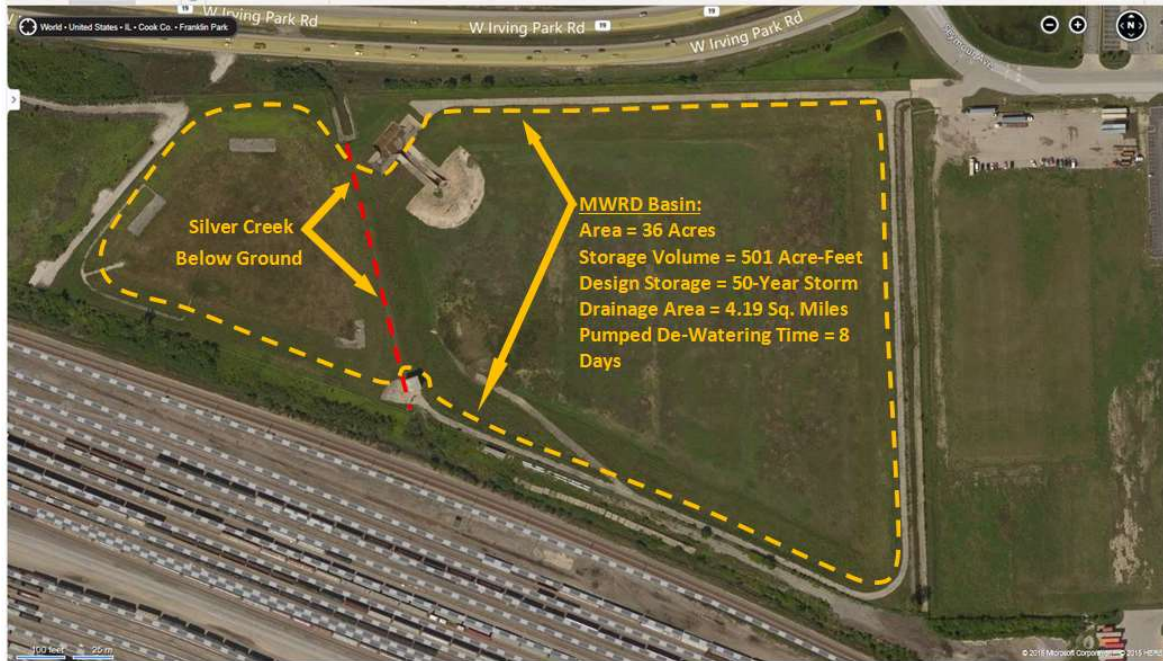
Photo 17: MWRD Flood Storage basin along Silver Creek located immediately south of O'Hare Airport (off Seymour Road). The MWRD Basin has an extensive runoff storage volume (501 acre-feet). However, Silver Creek is piped below ground (in a 60-inch culvert) over 700 LF along the site. Silver Creek overflows into the Basin (from the north) only during extreme flood events.
